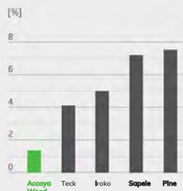
Accoya is suitable for coverings which, thanks to its dimensional stability, have a much longer lifespan and require less maintenance than other typical wood species.
